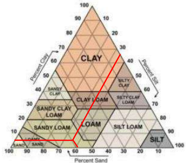
Figure 9. Soil analysis result – sandy loam
